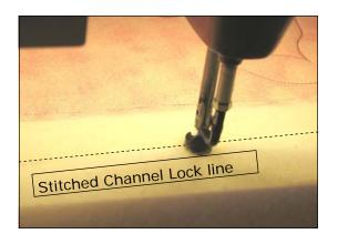
Leave the needle in the fabric and look at the pattern on the table. Notice where the light from the laser is located. The laser light should be on the lower horizontal registration line of the pattern. If the laser light is NOT on this line, carefully move the laser until it is on the line. See photos below.
