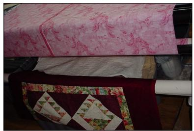
Gammill machines: Place the batting on top of the quilt backing fabric matching the approximate center of the batting and the center mark on the take up roller canvas and smooth batting flat. Do not stretch the batting.
